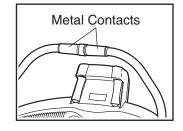
metal contacts on the handgrip pulse sensor, remove the plastic. If you use the chest pulse sensor and the handgrip pulse sensor at the same time, the console will not display your heart rate accurately.
